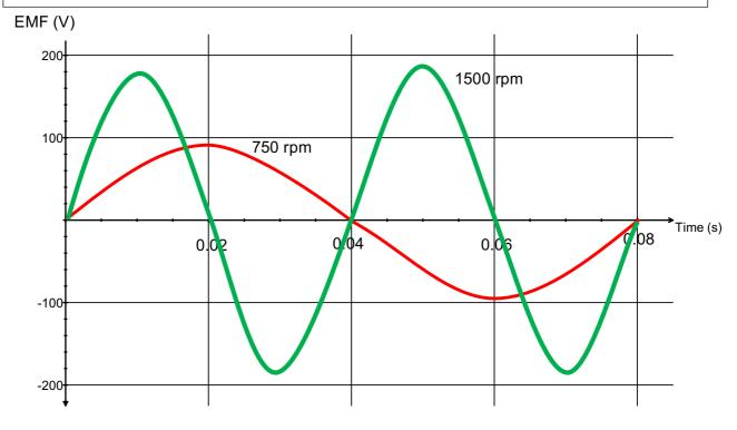
f) Sketch a second shape of the emf output for a rate of rotation of 1500 rpm and label this curve '1500 rpm'.
