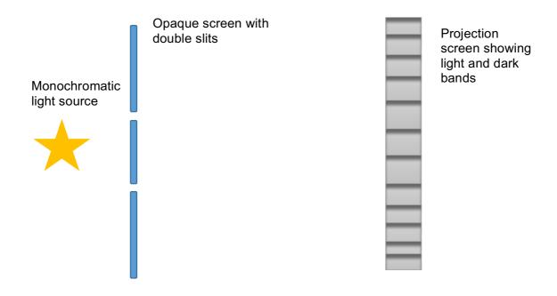
Light travels in waves and diffracts with circular wavefronts from each slit. ✓
