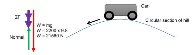
a) Construct a vector diagram in the box above. Show the forces acting on the car and the net force.
