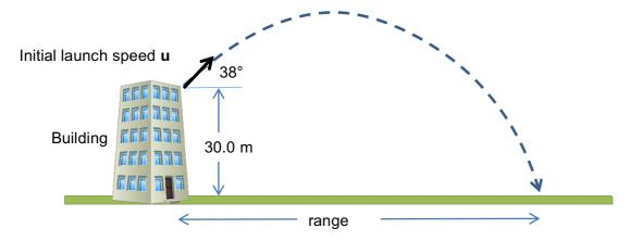
a) Calculate the initial launch speed  ${\bf u}$  of the stone.
